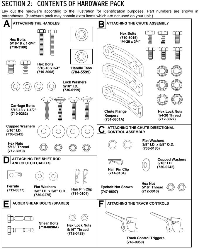
**NOTE:** The augers are secured to the spiral shaft with two shear bolts and hex lock nuts. If you hit a hard foreign object or an ice jam, the snow thrower is designed so that the bolts may shear. Two replacement shear bolts and nuts are provided for your convenience. Store in a safe place until needed.
